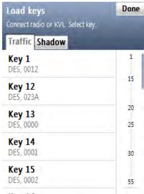
Figure 4-1 Load Keys Screen – Loading a Traffic Key (Example)
