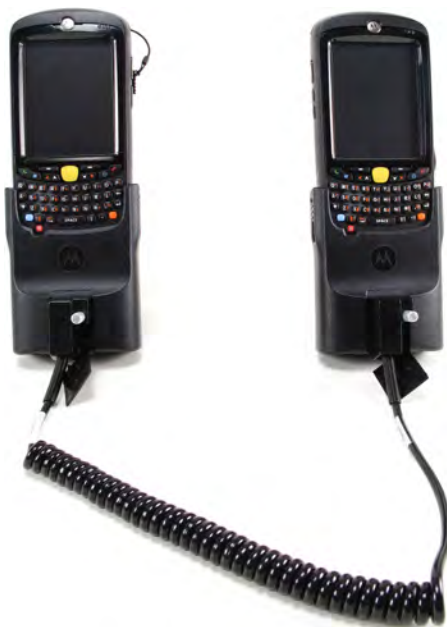
Figure 1-9 Two KVL Units – Connected
