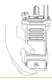
**4** Push at the bottom of the radio until the radio is released from it.
