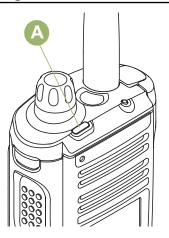
The Top Lightbar indicates the secondary function of MFK and also the status of Intelligent Lighting.
