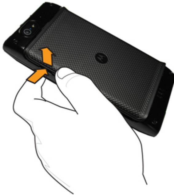
Figure 4: Removing the Battery Cover
