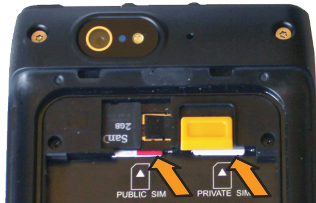
Figure 6: Installing the Public and Private SIM Cards
