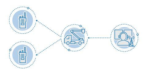
VRX1000-equipped vehicle extends simplex communications to portable radios from dispatch
