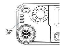
**NOTE**: The green LED lights up while the radio is transmitting and blinks rapidly when the radio is receiving a privacy-enabled call.
